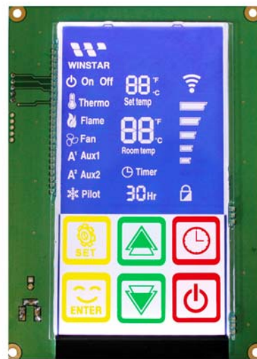
Winstar Single-layer Touch Key module with silk ink
